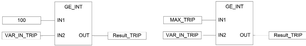
Fig. 16. An example involving the use of a literal as an input variable.
